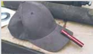
**Bob Payne, Coldwater, Miss.:** “When working under or inside a machine, visibility can be a problem - even in a well-lit shop. I’ve tried different kinds of strap-on lights and really like the Streamlight 66318 light, which clips onto the bill of a cap. It uses one AAA battery that lasts for a couple hours or more of continuous use. It’s great to have bright LED light right where you’re looking. You can buy it on Amazon.com for \$18.21 with free shipping.”
