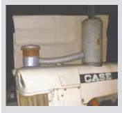
Ted Lacey, Hay Manager, Trent, S. Dak.: "You can make an air preheater for gas or diesel tractors by taking heated air off the outside of the muffler and directing it through a pipe to the air cleaner. The preheated air goes down into the carburetor, keeping it from icing up and preventing frost build-up. The photo shows the setup that's been on my Case 930 tractor for
