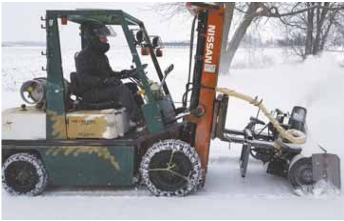
Paul Row came up with an inexpensive way to move snow by adapting an old 42-in. wide snowblower to his Nissan forklift. A cordless drill, controlled from the cab, is used to rotate the chute back and forth.
