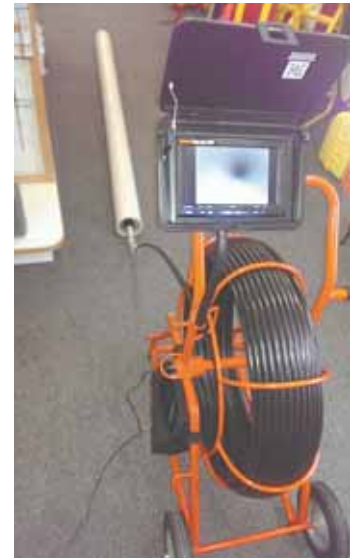
Do-it-yourself drain tile tools include digital locators, push rod transmitters, and push rod cameras.
