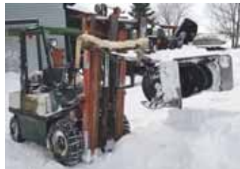
Row can tilt the snowblower up or down, or raise it 6 ft. high to remove the top of big snow drifts.
