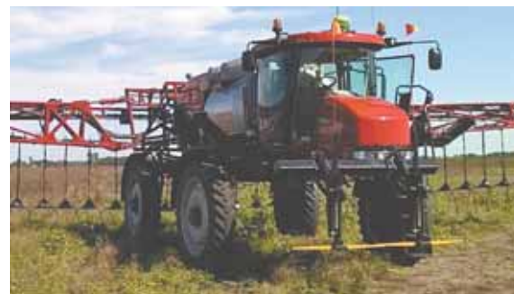
Flexible row sensors (yellow) mounted on front of this self-propelled sprayer steer the machine between rows, keeping it on course and preventing crop damage.
