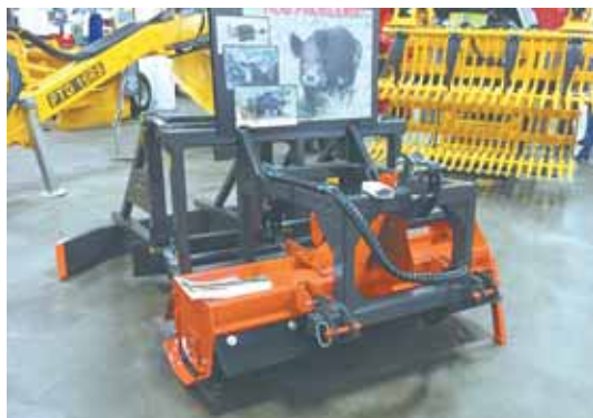
Hog Rooting Fixer comes with 3-pt. connectors for mounting a 60-in. reverse tine tiller to break up clods. A rear-mounted blade spreads them out.
