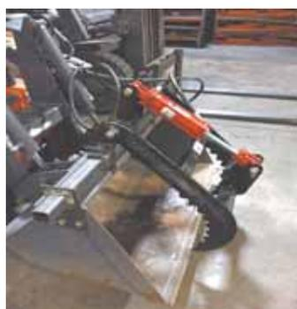
Kit comes with a 2-in. bore, 6-in. hydraulic cylinder.
