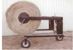
Tag-along cart (left) grabs round bales and lifts them off the ground. A hand crank is used to spin bale. Skid loader-mounted spinner uses a hydraulic motor with a chain drive.
