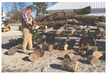
Brett Hundertmark cuts logs into firewood-size pieces using this mobile log deck. "I can stand while I saw, cutting logs between cross beams and letting them drop to the ground. Then I pull the wagon out of the way and split them," he says.
