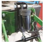
Electronic depth control kit for planters combines an electric actuator with a selfcontained hydraulic chamber.
