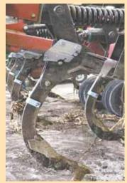
"Shear bolt monitor" lets you know right away when a shear bolt is broken so you can get that shank working again.
