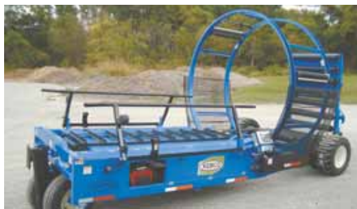
Kemco bale wrapper uses a web chain instead of a hydraulic cylinder to push bale forward.
