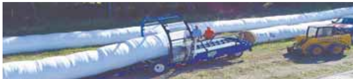
Placing bale on wrapper starts the chain. You can load the next bale without having to wait for a hydraulic cylinder to retract.
