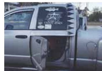
Sleeper bed replaces pickup's rear seat and extends about 8 in. beyond upper part of both rear doors. Bottom half of each door can still be opened and closed.
