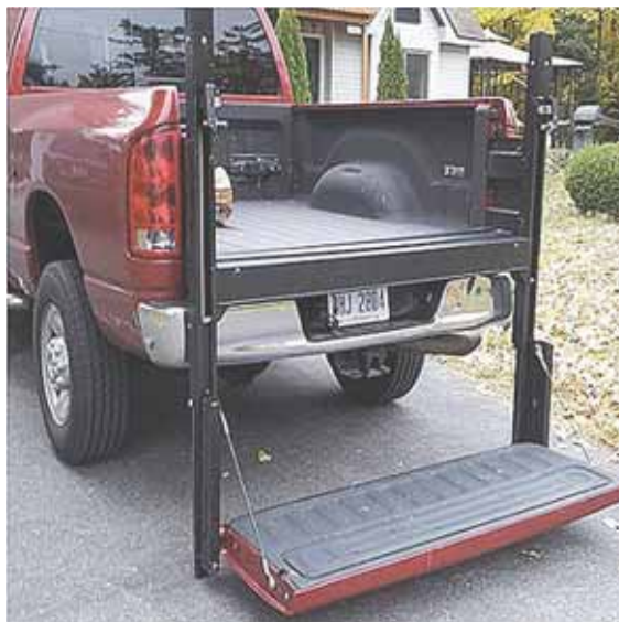
Electronic tailgate lift is designed to lift heavy tools and equipment while still allowing full use of existing tailgate.
