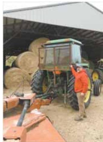
**Expanded metal rock guard helps keep flying rocks from breaking tractor cab's rear window.**
