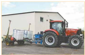
A-Cubed waterjet system equips planters and drills with waterjets instead of residuecutting coulters.
