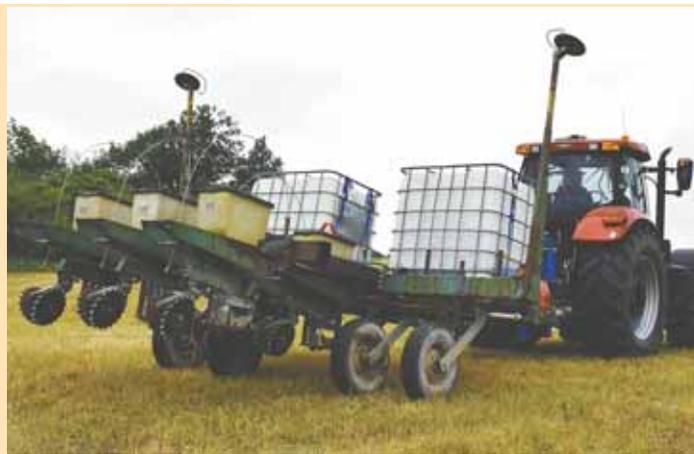
System cuts through crop residue and into the soil, using only 20 gal. of water or liquid fertilizer per acre.
