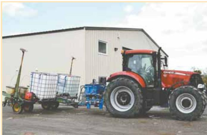
A-Cubed waterjet system equips planters and drills with waterjets instead of residue-cutting coulters.
