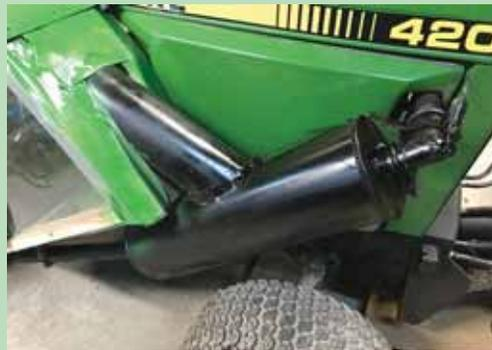
Heater consists of a 4-in. dia. muffler fitted inside a 6-in. dia. length of pipe. Heat captured from around the muffler is carried back into tractor's plexiglass cab, while exhaust fumes exit through a 2-in. dia. tailpipe that runs to back of tractor.
