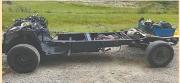
Winter cut the Prius unibody under the rear passenger seat and added a subframe (above). He then cut truck in two ahead of cab and overlaid the ends of the 2 frames. Removing the truck hood (right) reveals the Prius drive system.
