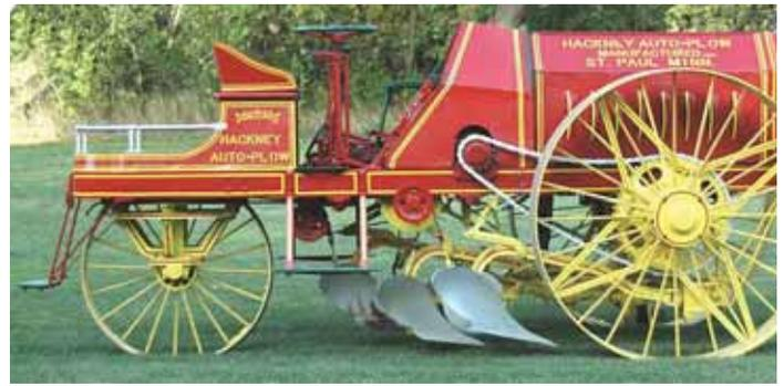
**Rare 1912 Hackney One Man Auto Plow has a pair of lugged steel wheels on front and a single steel wheel on back. A 3 or 4-bottom moldboard plow mounts underneath.**
