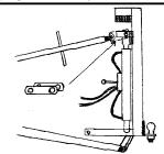
Drawing shows splitter in an upright position on tractor 3-pt. with ball hitch facing backwards. Starnes fashioned bracket to hook top link to splitting wedge.
