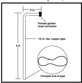
in the upper end and fitted it with a female garden hose fitting. The bottom end of the pipe is crimped. With just a little bit of water pressure, the pipe will dig itself into the
