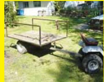
I build 2-wheeled yard trailers from old riding mowers by cutting off the back part of the tractor frame just ahead of the transaxle, keeping the rear tires and axle, and then welding a home-built 3 by 4-ft. deck on top of the frame and adding a hitch. Spacers keep the deck clear from the tires. I use a 4-wheeler or garden tractor to pull the trailer. The
