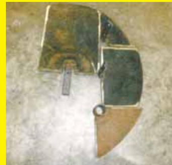
I want to share another idea I came up with several years ago to send to third world countries. I take an old 14 to 16-in. dia. disc blade and, with a plasma cutter, make 2 shovels and 6 garden hoes out of it. A short chunk of pipe can be welded on for attaching a wood handle. **(Ben Yantis, 2601 Lazy Days Lane, Sebring, Fla. 33872 ph 863 385-2378; yantisra@aol.com)**
