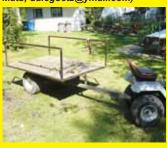
I build 2-wheeled yard trailers from old riding mowers by cutting off the back part of the tractor frame just ahead of the transaxle, keeping the rear tires and axle, and then welding a home-built 3 by 4-ft. deck on top of the frame and adding a hitch. Spacers keep the deck clear from the tires. I use a 4-wheeler or garden tractor to pull the trailer. The
