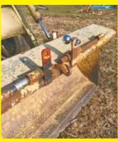
I modified my Ford 4000 front loader bucket so that it has both a ball hitch and a pin hitch on top, along with a chain hook. To use the hitches I just tilt the bucket forward. Pushing a trailer into a storage building is a lot easier than trying to back it in. (Larry Wood, lawpressman@aol.com; ph 740 360-
