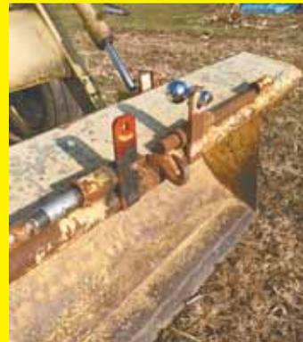
I modified my Ford 4000 front loader bucket so that it has both a ball hitch and a pin hitch on top, along with a chain hook. To use the hitches I just tilt the bucket forward. Pushing a trailer into a storage building is a lot easier than trying to back it in. **(Larry Wood, lawpressman@aol.com; ph 740 360-1956)**
