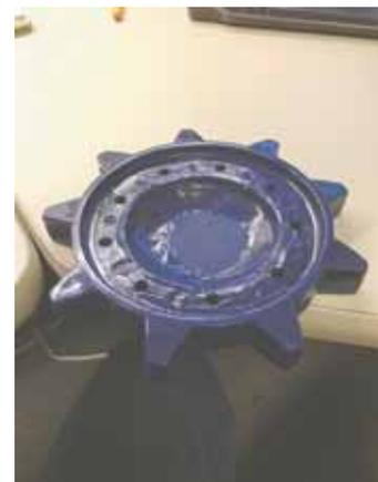
**Plan Tech uses a split-mold method to make cast polyurethane drive and gear sprockets. “Parts we produce are twice as good as injection molding in terms of tensile strength and compression,” says Kevin Healy.**
