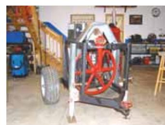
**Generator mounts on a home-built 2-wheeled trailer (small pulley shown near fan drive pulley is not used to operate generator).**
