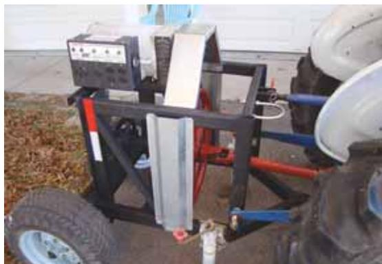
**Don Prestien used the fan drive pulley and pto shaft off an old portable grain dryer to turn an old engine-driven, 10k generator into a pto-driven unit.**
