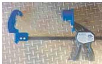
**Two-piece clamp is equipped with a “hook” at one end and a trigger-type handle at other end, making it easy to align replacement parts properly.**
