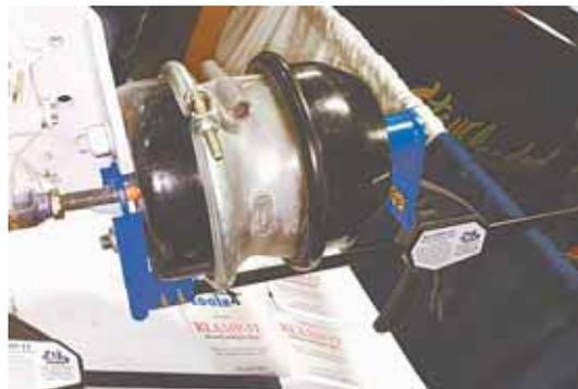
**Klamp-It Brake Service Tool makes it easy for one person to change the brake diaphragms right on a truck.**
