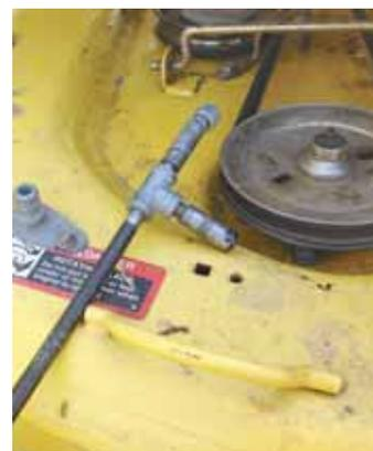
**Another grease fitting is threaded onto far end of T. Galde caps it off when using the other fitting.**
