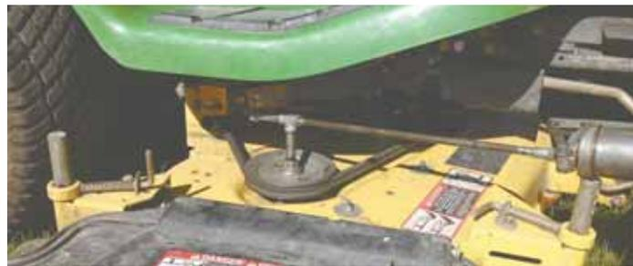
**Marlin Galde replaced the tube on his grease gun with a 15-in. straight pipe extension, making it easier to lubricate the deck pulleys on his riding mower. A T fitting is threaded onto end of pipe, and a grease fitting threaded onto bottom of T.**
