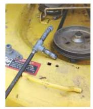
Another grease fitting is threaded onto far end of T. Galde caps it off when using the other fitting.
