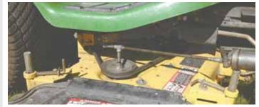
Marlin Galde replaced the tube on his grease gun with a 15-in. straight pipe extension, making it easier to lubricate the deck pulleys on his riding mower. A T fitting is threaded onto end of pipe, and a grease fitting threaded onto bottom of T.
