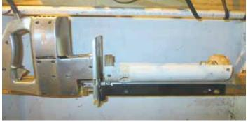
Wall-mounted, automatic paint can "shaker" uses a 10-in. length of pvc tubing cut in half lengthwise and attached to an old sabre saw.
