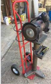
**Bob Payne, Coldwater, Miss.:** "I bolted my stationary grinder onto an inexpensive 2-wheeler cart so that I can move it around wherever there's good light and ventilation. The cart also makes the grinder easy to store out of the way. The base attaches to the foot of the 2-wheeler with 2 big bolts and washers."
