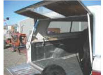
When the rear door lift cylinders on his pickup topper failed, Jeff Hoard replaced them with pieces of pvc pipe. Notch cut into lower end of pipe slides into tailgate’s latch catch.
