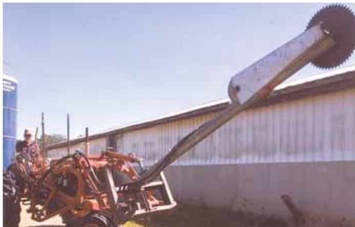
Boom on loader-mounted tree shear is fitted with a 20-in. blade that’s belt-driven by a hydraulic motor.
