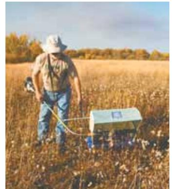
Hand-held seed harvester is powered by a heavy-duty line trimmer that operates parallel to the ground. It spins an 18-in. reel that grabs seeds and throws them into a hopper bag.
