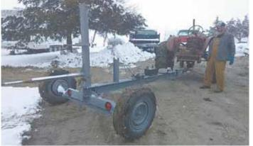
Trailer-mounted bale spear sticks out the back and pivots forward using a winch and pulley system.
