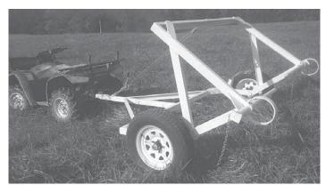
Ground-driven, single bale round bale unroller can be used to feed cattle without tearing up the ground, and without the expense of a tractor. a tractor.'
