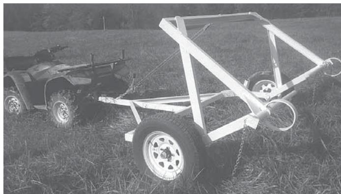
Ground-driven, single bale round bale unroller can be used to feed cattle without tearing up the ground, and without the expense of a tractor.
