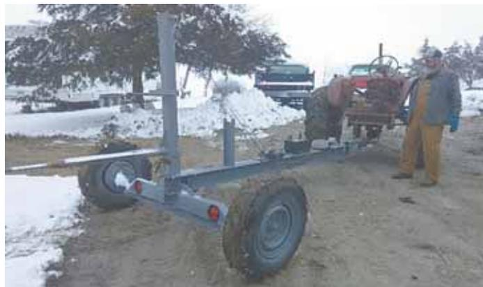
Trailer-mounted bale spear sticks out the back and pivots forward using a winch and pulley system.
