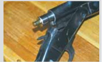
**Rifled adapters that fit into shotgun barrels make it possible to shoot smaller caliber ammo with the same gun.**
