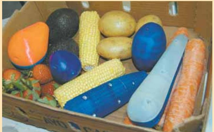
Battery-powered, data-gathering cases are shaped like the produce being monitored.
