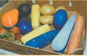
Battery-powered, data-gathering cases are shaped like the produce being monitored.
