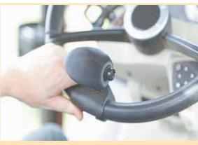
Mini thumbcontrolled joystick at one end of mouse is used to control loader operations.
