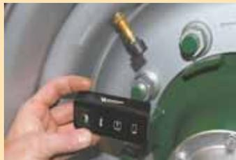
Pressure sensor caps screw onto valve stems and send alerts to a small handheld monitor if tire pressure drops.
