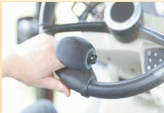
Mini thumb-controlled joystick at one end of mouse is used to control loader operations.
