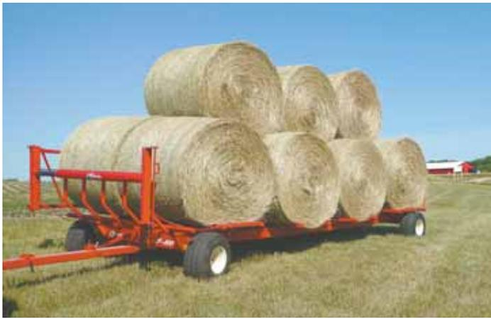
E-Z Trail's big bale wagon carries round or big square bales and quickly converts to a portable feeder by adding removable side panels.
