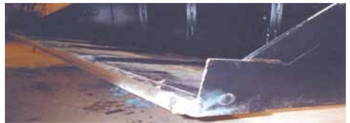
Solid steel shaft is attached to front edge of loader bucket. It's held in place by square steel plates welded to each end of bucket and 3 pieces of 1-in. sq. tubing.
