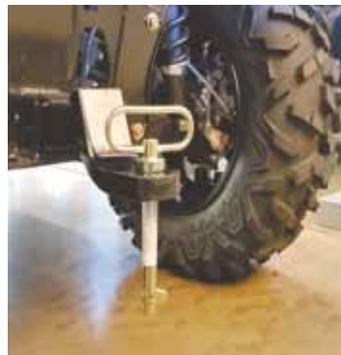
Latch near bottom of hitch pin automatically locks itself, eliminating the need for cotter pins.
