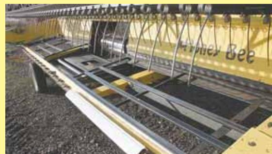
Cutter Cap comes in 5-ft. sections and snaps onto sicklebar knife guards to protect from accidental cuts.
