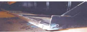
Solid steel shaft is attached to front edge of loader bucket. It's held in place by square steel plates welded to each end of bucket and 3 pieces of 1-in. sq. tubing.
