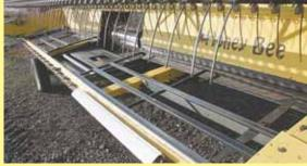
Cutter Cap comes in 5-ft. sections and snaps onto sicklebar knife guards to protect from accidental cuts.
