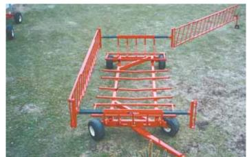
Panels slide out to an 11-ft. width when trailer is loaded, and then slide in to a 5 1/2-ft. width as cattle press toward the center while feeding.
