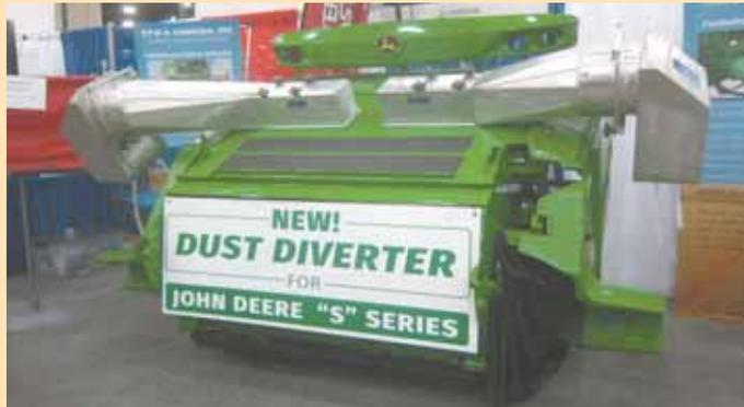
Hydraulic-powered dust diverter for Deere "S" series combines mounts directly over the feederhouse door, discharging dust down both sides.
