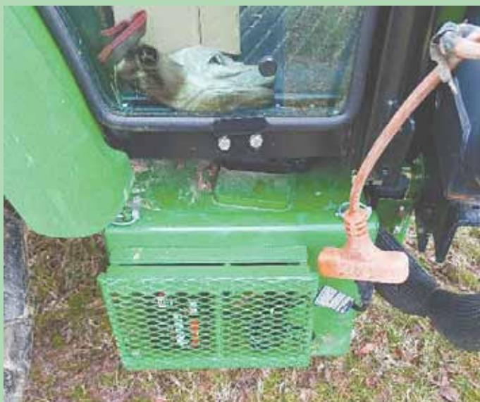
**On-board charger hooks up to tractor's battery box and is covered by a metal cage. To charge the battery, Jett pulls out charger cord pigtail and hooks it up to an extension cord.**
