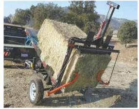
Hydraulicoperated blade on back slices down through bale to feed it out one flake at a time.
