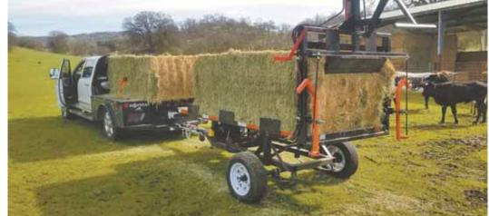
Flaker/feeder is designed to feed 3 by 3-ft. or 3 by 4-ft. big square bales. It comes with an electric winch that can be used to load the bale onto the trailer after the first bale has been fed out.
