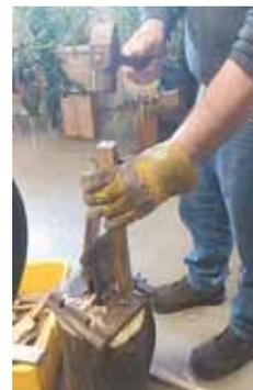
An ax head is welded to the top of a heavy steel plate which is then bolted to a log.
