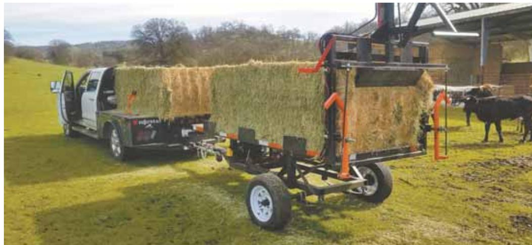
Flaker/feeder is designed to feed 3 by 3-ft. or 3 by 4-ft. big square bales. It comes with an electric winch that can be used to load the bale onto the trailer after the first bale has been fed out.
