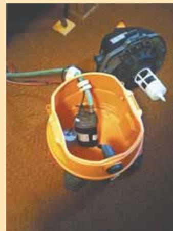
Small sump pump fits inside shop vac and has a 100-ft. hose attached to it. As the vac fills with water, the float switch activates the sump to empty it.
