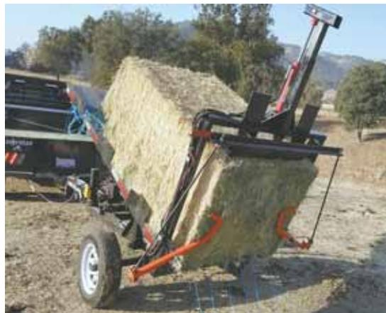
Hydraulic-operated blade on back slices down through bale to feed it out one flake at a time.
