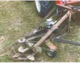
Schild built this fenceline mower out of an old walk-behind mower, stripping it down to the frame, wheel mounts, and 20-in. mower blade assembly.
