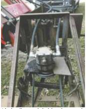
A hydraulic pump belt-drives the mower in place of the walk-behind mower's engine.
