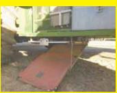
Thank you for featuring our low-cost Bin Buster drop pan for combines that collects chaff and straw coming out of the combine to measure grain loss. It's made from a tarp stretched over fiberglass rods, which makes it flexible so the combine wheel can run over it. There are two videos showing how it works at farmshow.com or on FARM SHOW's YouTube channel. If you're interested in buying one, get your order in early
