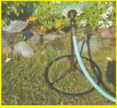
I welded this nozzle holder together using an old tractor steering wheel, a length of 1/2-in. dia. steel pipe, and a 3/4-in. washer. It's so handy I made two, one for the front yard and one for the back. The flowers benefit from the showers and the rainbows they make seem to attract hummingbirds. It's a nice way to spot spray the gardens around my home. (Rich Peterson, Plymouth, Wis.)
