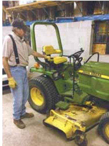
Mark Rinke says changing out the seat, lengthening the steering wheel, adding grab bars, and new side steps make his Deere 855 tractor easier to get on and safer to use.
