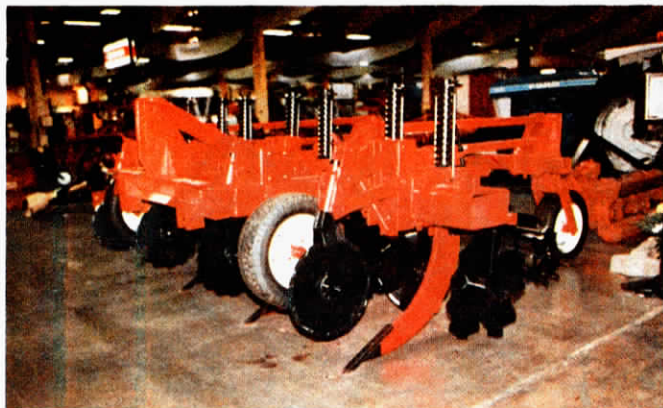
The 3 pt. mounted Ro-Till is available with a pull or lift hitch for trailing conventional pull or mounted planters.
