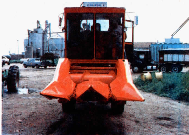
Custom combine, built with a cab for two, features adjustable (from 30 to 40 in.) row width.
