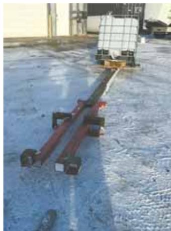
Skid loader forks fit inside square tubing pieces welded to a steel frame.
