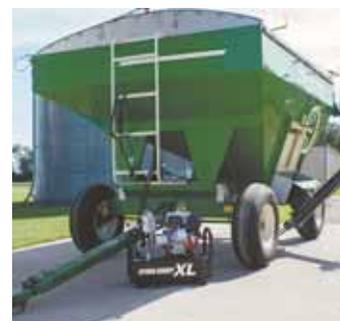
Small engine-powered portable hydraulic packs produce enough power to operate everything from augers to log splitters.
