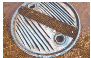
Bryan cut off the top 3 in. of a plastic barrel and then made a series of long parallel "louvers" in the lid.
