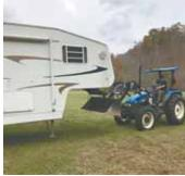
Short steel pipe welded on top of bucket forms a "cup" to lift camper's king pin.
