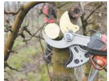
Cutting through wood up to 2 1/4 in. dia. is easy with this new electronic pruning shears.
