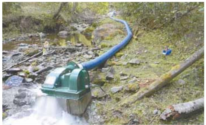
Low-head hydropower, cross-flow turbine generator "works like a squirrel cage made of stainless steel", says inventor Bill Scott.
