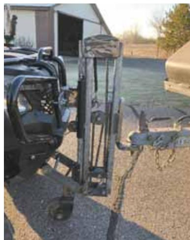
Dave Sand can easily move trailers using this unique front hitch that he built for his ATV. An electric winch provides lift.
