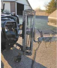
Dave Sand can easily move trailers using this unique front hitch that he built for his ATV. An electric winch provides lift.
