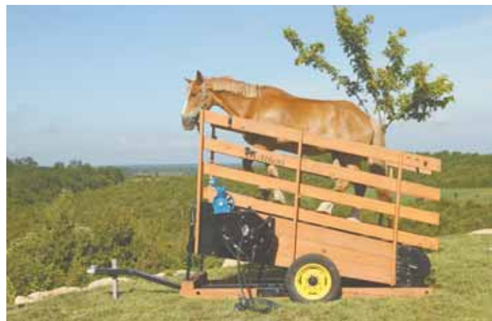
Horse-powered treadmill can be used to power everything from wood splitters to water pumps.
