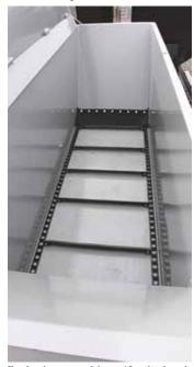
Feeder is powered by a 12-volt electric motor that drives a floor chain through a 50-to-1 gearbox.
