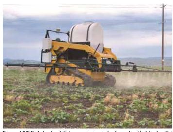
Dave and Bill Farb developed their own autosteer technology using this driverless Cat Track Loader, which can "communicate" with any pull-type or 3-pt. implement.
