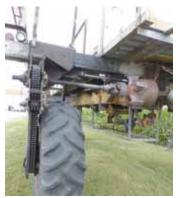
Back end of spreader was replaced with the rear end from a Chevy truck and the mechanical final drive system from a Deere
