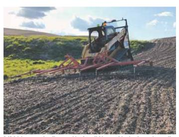
Self-driving tractor handles everything from disking to cultivating, harrowing, seeding, and spraying. Software pairs machine's control system with GPS guidance.
