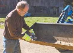
A handheld grinder can be used to sharpen the edge on a tractor's loader bucket, making it easier to use the loader to take out groups of problem weeds. It also helps with digging.
