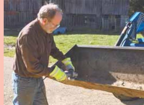
A handheld grinder can be used to sharpen the edge on a tractor's loader bucket, making it easier to use the loader to take out groups of problem weeds. It also helps with digging.
