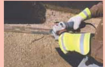
Bucket's leading edge is sharpened to a knife's edge.
