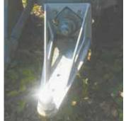
Home-built ball hitch extends back 18 in. and bolts on around Ford 9N's pto shaft.
