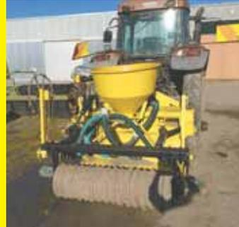
One of my horticultural clients designed and built this 3-pt. mounted, 5-ft. wide seeder for permanent bed farming. It features a 150 hp. gearbox, two 20-in. long in-bed rippers, two wheel track rippers with inward-facing deflectors, a large capacity hopper for seed or fertilizer, and two different distributors. A 12-volt fan is used to apply the fertilizer or seed.
