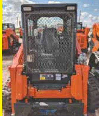
Thanks for the article on my screen guards designed to protect tractor cab windows as well as the tractor operator (Vol. 42, No. 4). I recently built a guard for skid loaders used in the forestry business. The photo shows it mounted on front of a Kubota 95 SVL skid loader. Protecting the front window and the operator from wood debris is the goal of this screen. The guard is installed with just 4 bolts, which go through 1/4-in. "ears" on each side of the screen.
